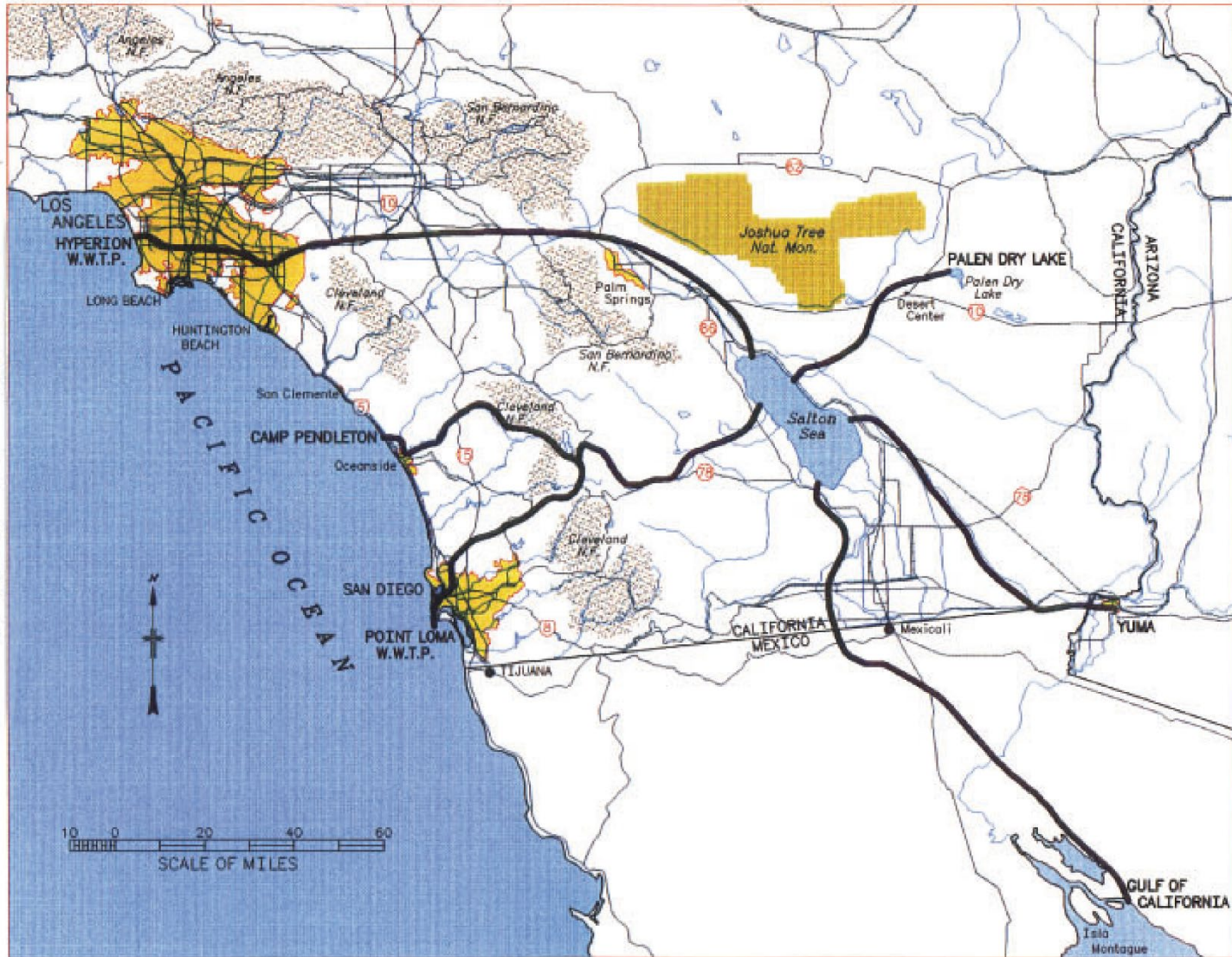
Figure 13.—Pipeline routes to and from Salton Sea.
